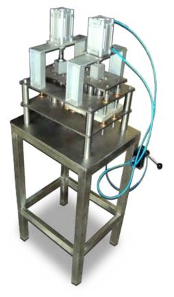
This device is pneumatically operated; feeding of sheet is manually done. The punched items discharge onto a tray below.
